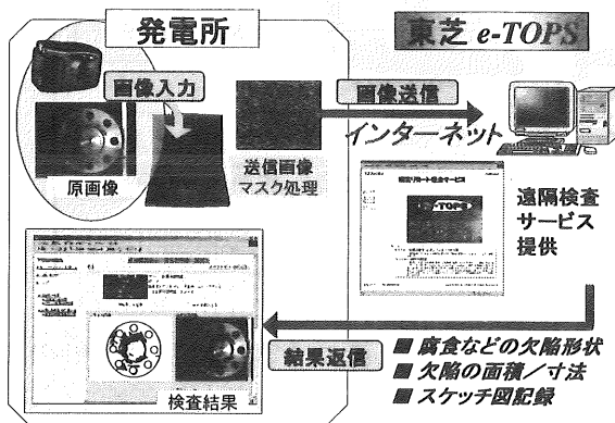
Fig. 5 Outline of remote inspection service system applied Image processing technologies
