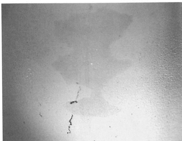
Fig.5 Typical example of PT indication after removing the cracks by grinding
