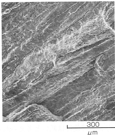
Fig.9 SEM observation on fracture surface in a scoop-sample
