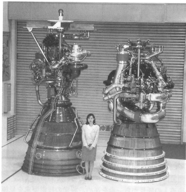
Fig.1 LE-7/A Engine for H-II/A 1st stage
