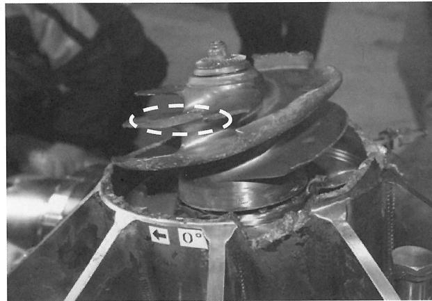
Fig. 3 broken hydrogen inducer
