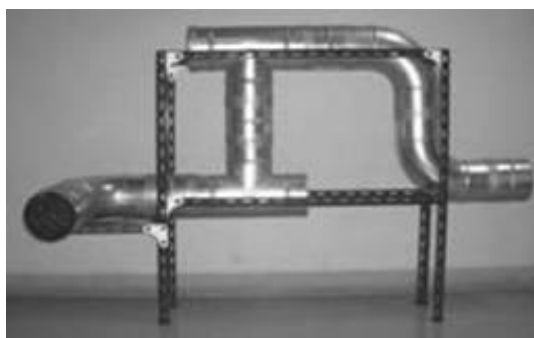
Fig.13 Geometry of piping used in the experiment.
