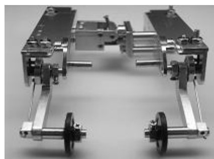
Fig.6a Attachment which gives the restoring moment to the robot.
