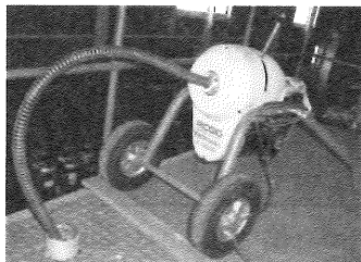
Fig.4 Blockage clearing equipment
