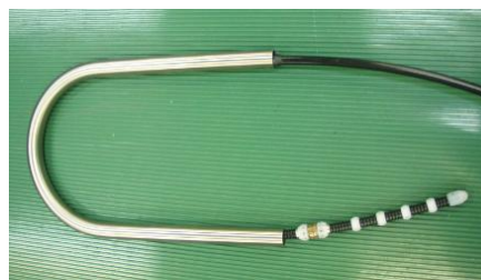
Fig. 5 Passing Probe through Small U-bend (Y1)
