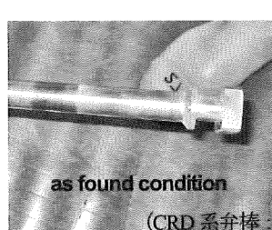
Fig.7 Surface appearance of CRD valve stem
