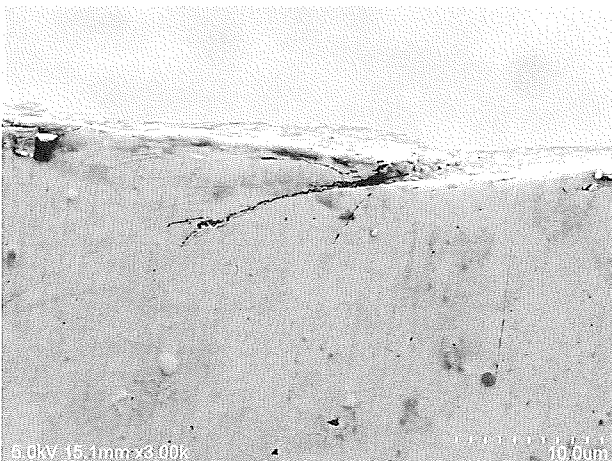
Fig. 5 SEM micrograph of crack observed in nickel base alloy weld metal as shot peening.
