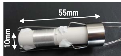
Fig.10 Structure and appearance of the hydrogen sensor for experiments
