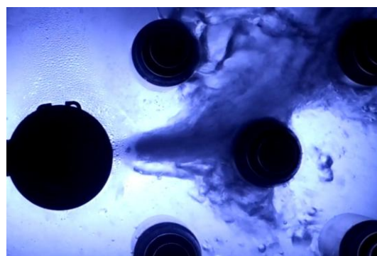
(b) Steam jet in subcooled water at T=95℃
