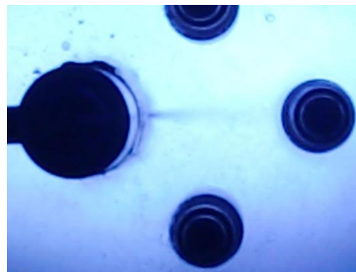
(a) Steam jet in subcooled water at T=50℃
