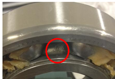
Fig.3 Slit shaped damage (Test D2: Bearing 6312)
