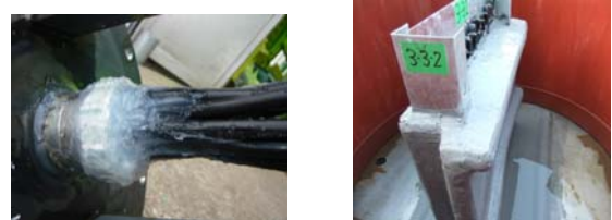
Fig.2 Photographs of test equipment (left: conduit, right: cable tray)
