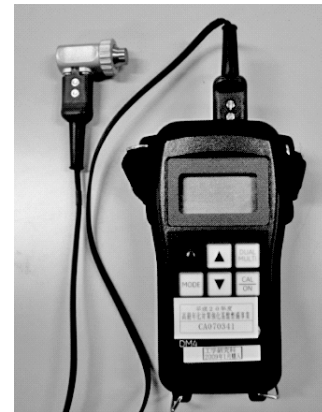
Fig.6 Ultrasonic thickness gauge.
