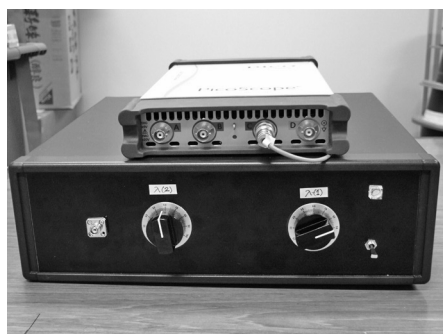
Fig.4 FBG-OTDR system with digital oscilloscope (upper)
