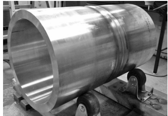
Fig. 2 Appearance of butt welded stainless steel pipe.
