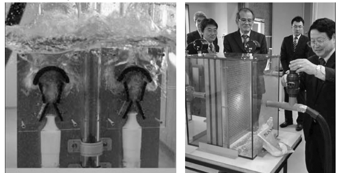
(a) Modified venturi scrubber (b) Metallic fiber filter Fig.8 Fundamental visualized tests for wet and dry filter
