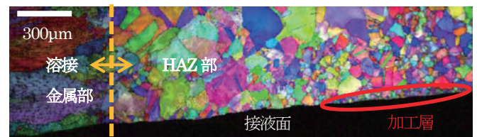
Fig.6 Crystal orientation of Heat affected zone
