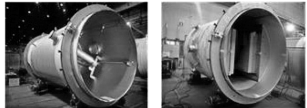
Fig.10 Manufacture of Filtered Venting Equipment (Venturi scrubber, Metal fiber filter)
