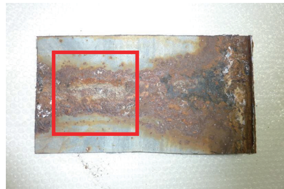
Fig.4 Ultimate analysis (Outer surface of the side plate)
