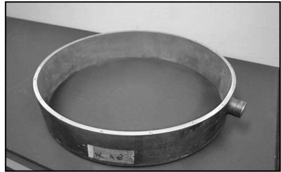
Fig.2 Photographs of the appearance of the Monju secondary cooling system pipe that was removed from the plant
