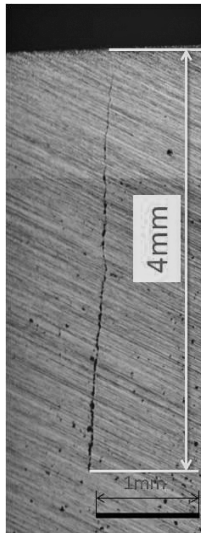
Fig. 4 Fractography of crack of stress cycle 265,000
