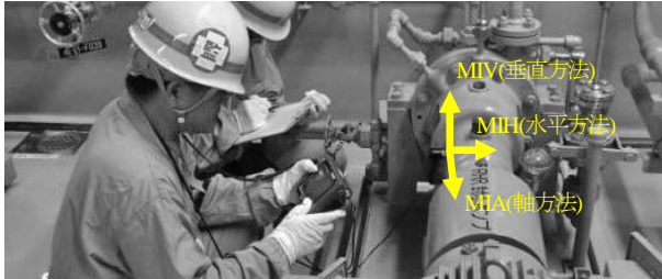
Fig.2 Picture of vibration monitoring
