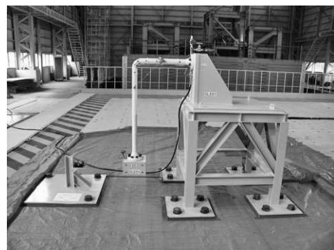
Fig.4 Piping elbow specimens under seismic loadings [6]
