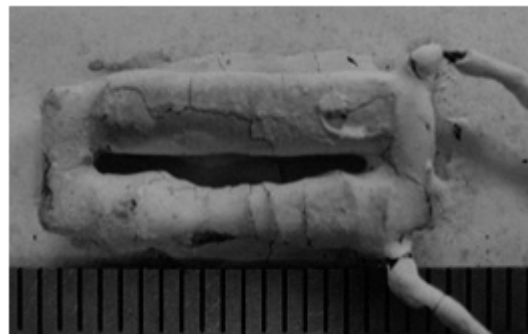
Fig. 12 Photograph of a magnetic sensor element using Permendur magnetic core after a performance evaluation test
