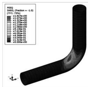
Fig. 9 Elbow1 outer face equivalent plastic strain
