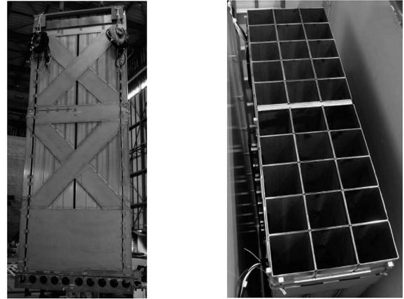
Fig.4 The Test Fuel Rack (Square Tube Type)
