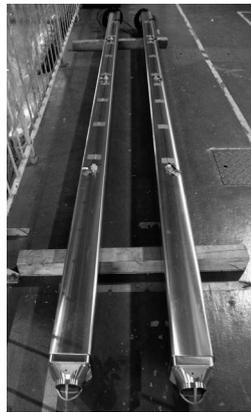
Fig.3 The Simulant Fuel Assembly (Right : Simplified, Left : Detailed)
