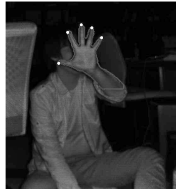
Fig.8 Result of stretched fingertips detection in real time
