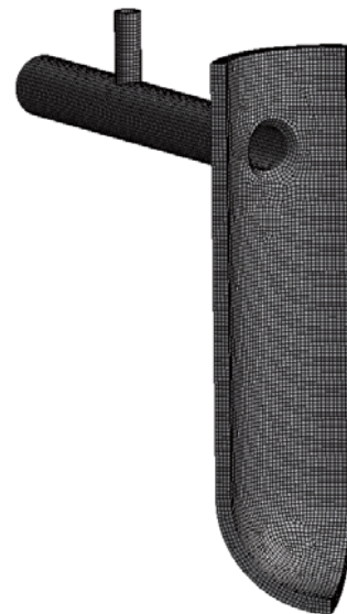
Fig.5 RPV mesh of the mechanical model.
