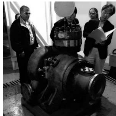
Fig.8 Hydraulic Test (Confirm of Pressure Gauge)
