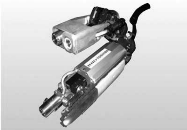
Fig. remote controlled robot for internal primary containment vessel PC investigation
