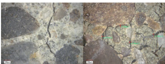
Fig. 8 Comparison of specimen (400°C and 1100°C)
