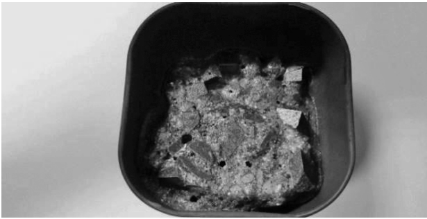
Fig. 3 Molten specimen (1200°C)
