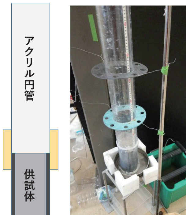
Fig. 2 Permeability measurement devise
