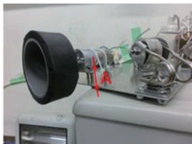
Fig.6 Drive wheel installation height
