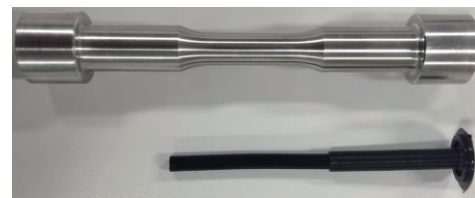
Fig.2 Hollow specimen and 3-dimensional replica
