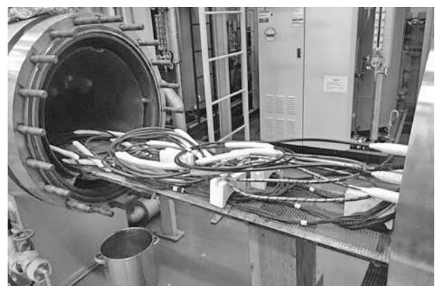
**Fig. 3 SiR and FR-EPDM cables and a steam exposure chamber before the steam exposure of condition 1 (155 °C, 0.444 MPaG, 336 h).**
