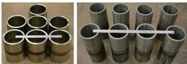
(a) Same welded joint (b) Dissimilar welded joint
