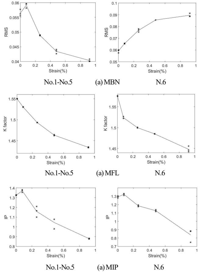
**Fig.2 The relationship between NDT signals and strains**
