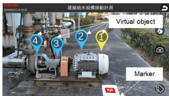
Fig.7 Support of sensor attachment
