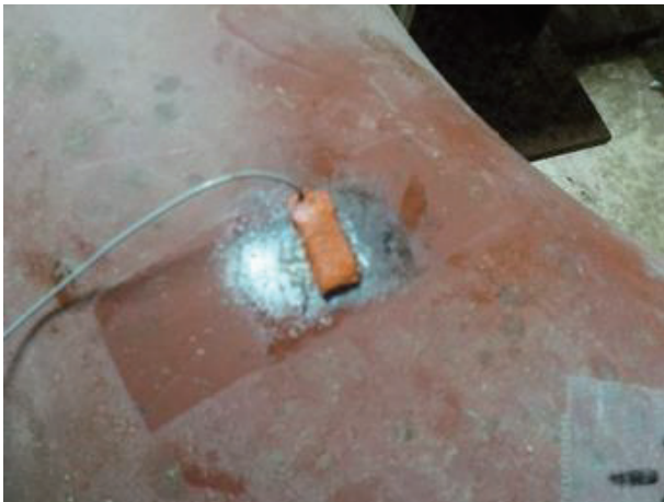
Fig.4 FDUTM attached on the test location
