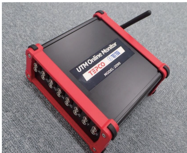
Fig.2 Appearance of UTM online monitor
