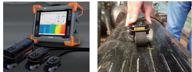
Fig.1 Appearance of Pulsed Eddy Current device [1] and pipe wall thickness measurement
