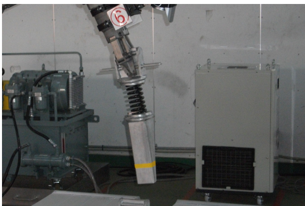
Fig.3 Mock-up of new rubble removal tool
