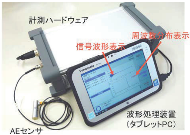
Fig. 3 AE Hammering inspection system
