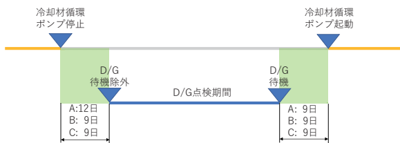
Fig.5 Preparation period for D/G inspection
