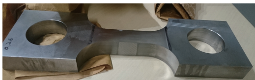
Fig.3 Tensile test specimen used in this study
