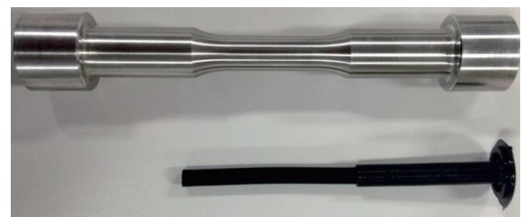
Fig.2 Hollow specimen and 3-dimensional replica
