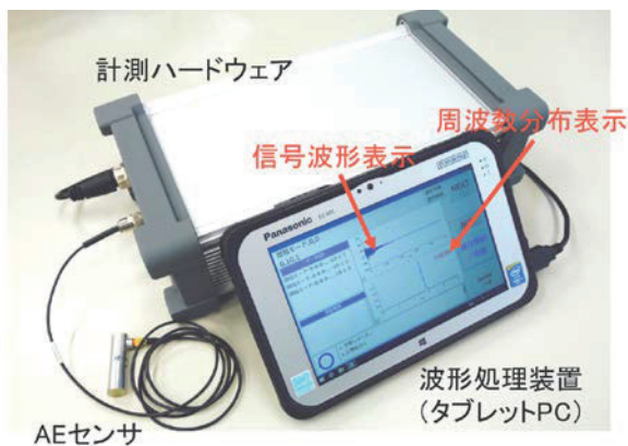
Fig. 4 AE Hammering Inspection system
