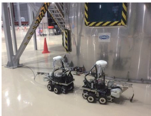
Fig.1 Demonstration of an Optical Fiber Vibrometer Installation by a Prototype Robot at a Water Tank of the JAEA-NARAHA Center
