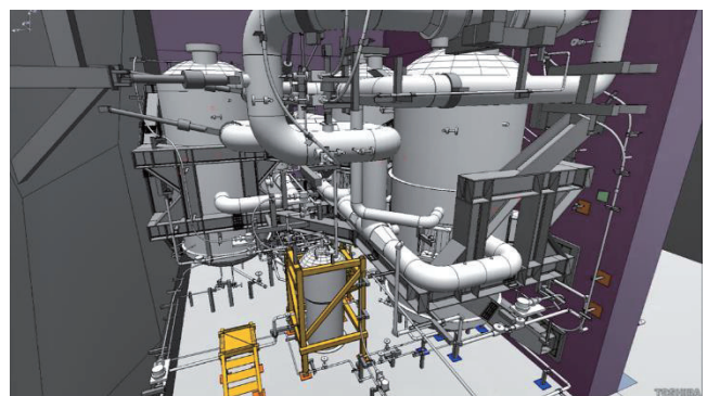
Fig.5 Completion image of FCVS installation
