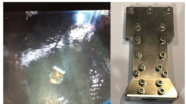
Fig.27 Steam test at Okano Valve for scrubber nozzle.
