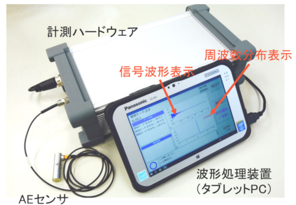
Fig. 3 AE Hammering Inspection system
