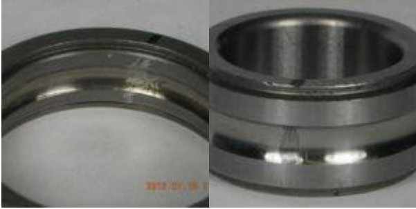
Fig.3 Bearing components in the MFPS dataset: (left) outer race failure and (right) inner race failure [6].
